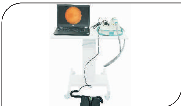
Shishunethra, which is a portable, handheld, lightweight, easy to use, ROP screening device to screen pre-mature babies in India has been developed by Forus Health Pvt. Ltd., Bengaluru
