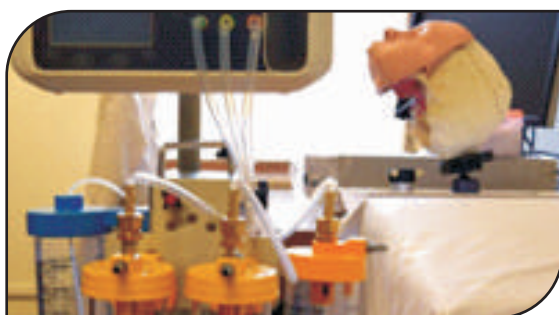
A device for secretion and oral hygiene management to reduce risk of acquiring ventilator associated pneumonia developed by Coeo Labs Pvt Ltd, Bengaluru
