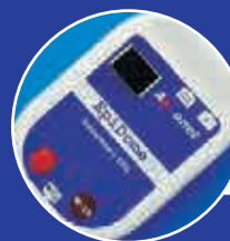
An affordable ambulatory EEG device developed by Axxonet System Technologies in collaboration with NIMHANS, Bangalore
