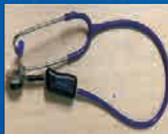
Device to convert conventional stethoscope into digital stethoscope
