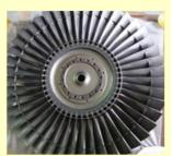
Detonation Spray Coated LPC III modules for Naval Aircraft
