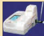
PoC Diagnostic- disease detection system developed for Malaria, Dengue and Typhoid
