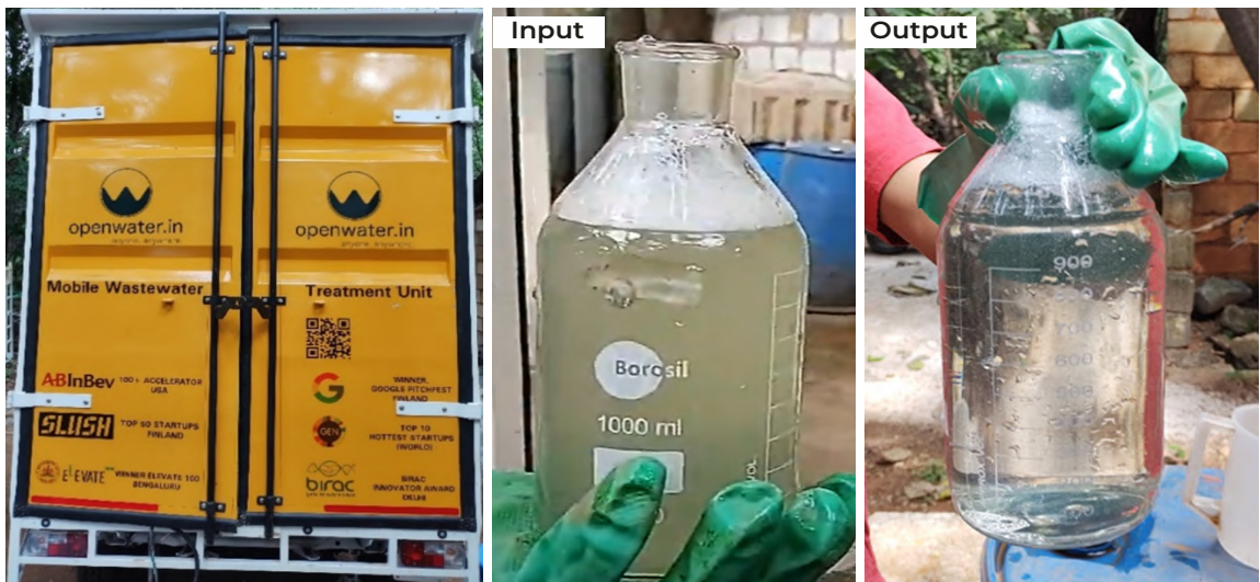
Membraneless, chemical free, wastewater treatment system (Openwater.in, Bengaluru)
