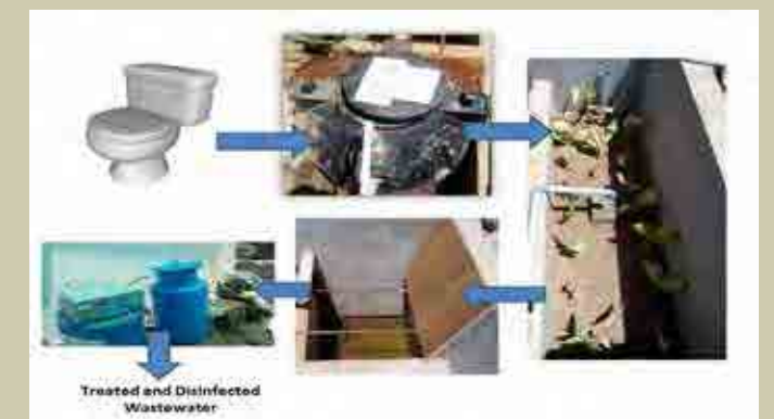
Electrochemical vector connected to a septic tank for a single toilet
